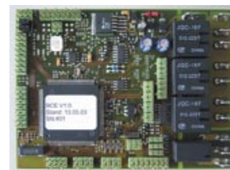
BCE control unit.
