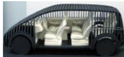
1:4 Foam model for representing a variable interior concept.
