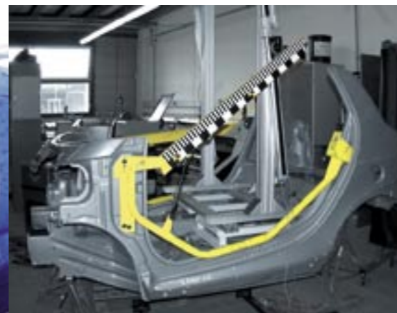
Door bar endurance test on a special test rig developed and built for this purpose.
