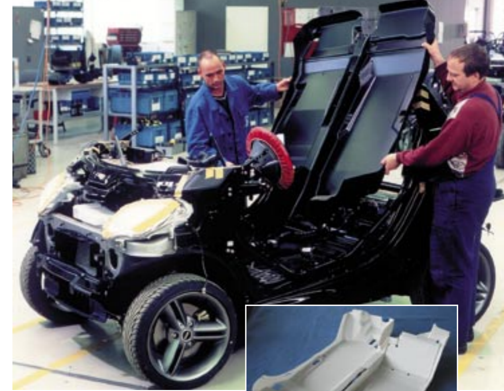
Floor compartment in SLS as a 1:4 model and as a trimmed moulding on installation.
