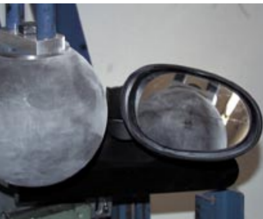
Outside mirror test: Does the mirror fold in on impact in accordance with the regulations?
