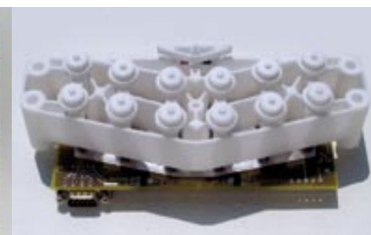
Control panel supports and boards.
