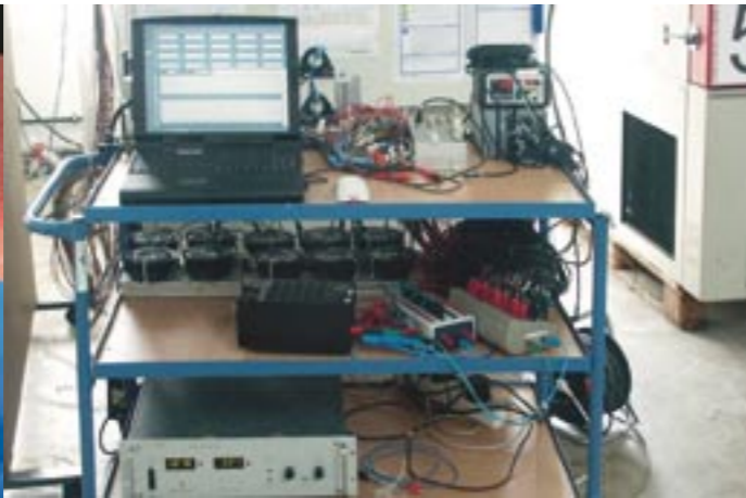
Electric test structure for long-term system testing in a climatic test environment. Computer-based control and visualisation environment including constant monitoring and recording of data.
