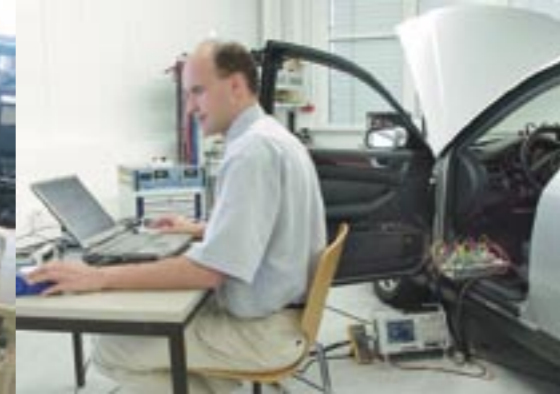
System tests in a networked cluster (CAN, LIN, MOST) on a vehicle system simulator and on a LabCar.
