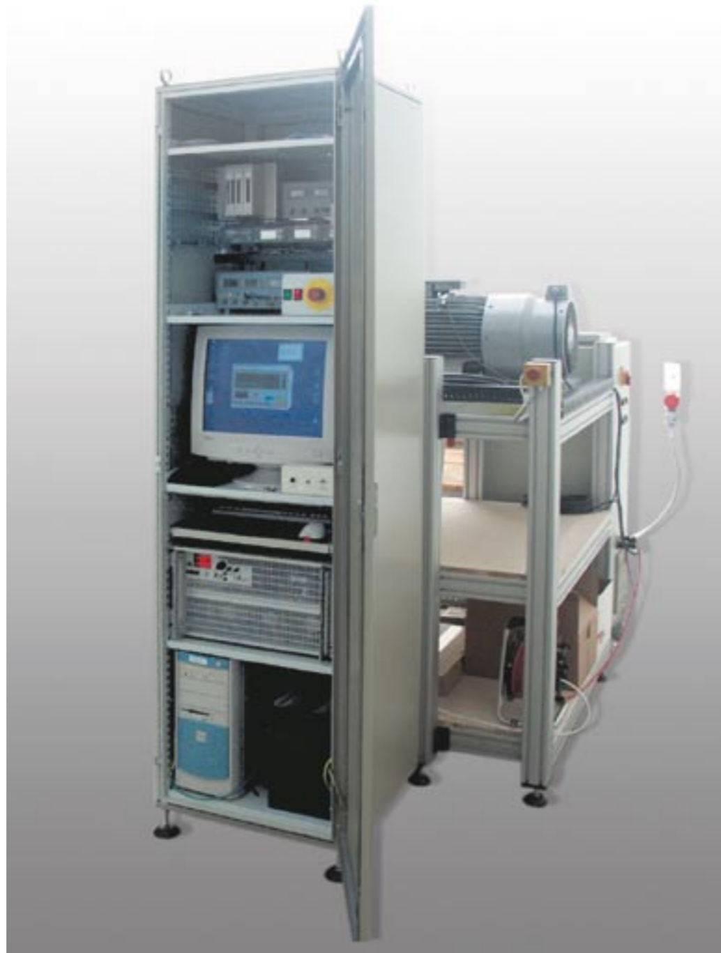
Test bed for vehicle electrical systems, used to evaluate system functions.
