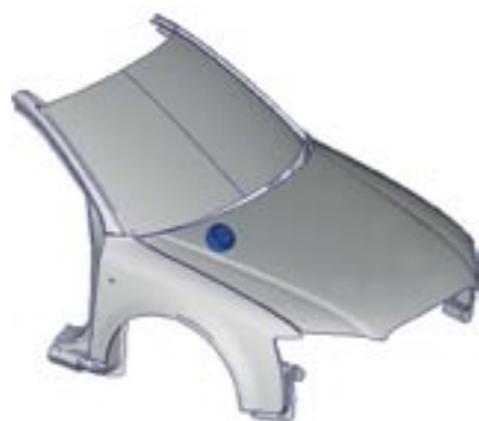
Front-end structure of the Audi A4 with the Head-Form-Impactor.
