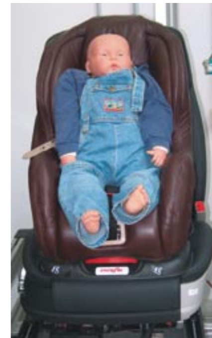
Child seat with dummy representing one year old on the seat test bench.
