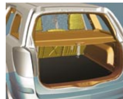
The luggage compartment cover in the Astra estate with easy opening concept.
