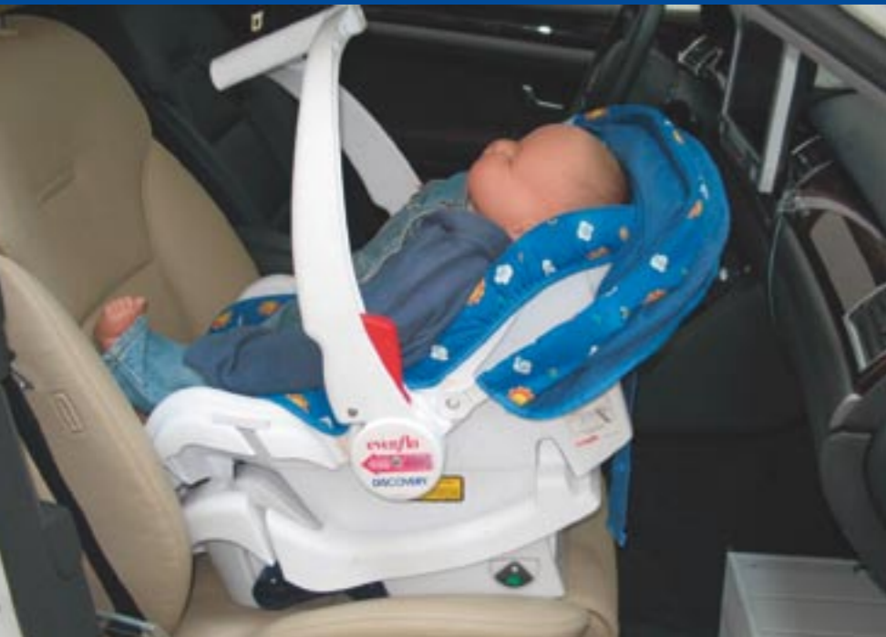
Rear-facing child seat mounted on the passenger seat. In the USA the automatic airbag deactivation must be warranted in future.
