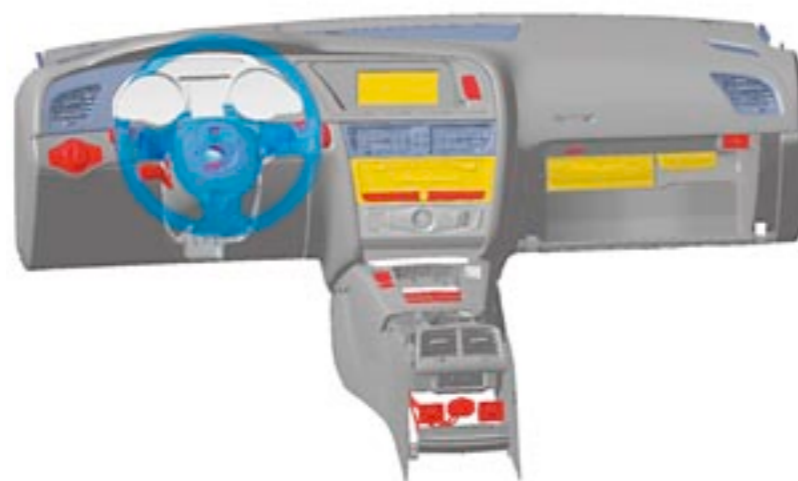
The isometric representation of the CAD model of the cockpit with the centre console.
