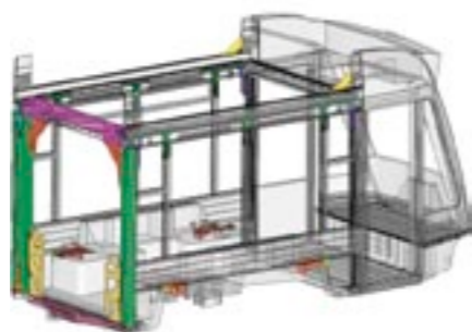
The new solution involved using sheet-metal parts, extruded parts, cast parts and forged parts to reinforce the structure.
