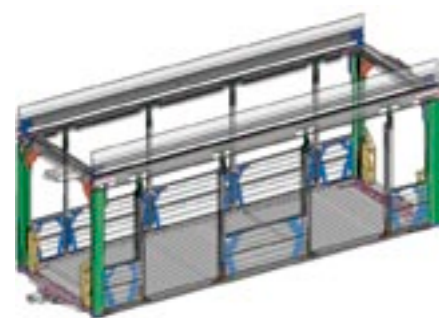
The new solution involved using sheet-metal parts, extruded parts, cast parts and forged parts to reinforce the structure.
