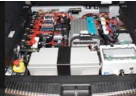
Energy management system in the spare wheel well of the Valeo Comfort Demo Car.
