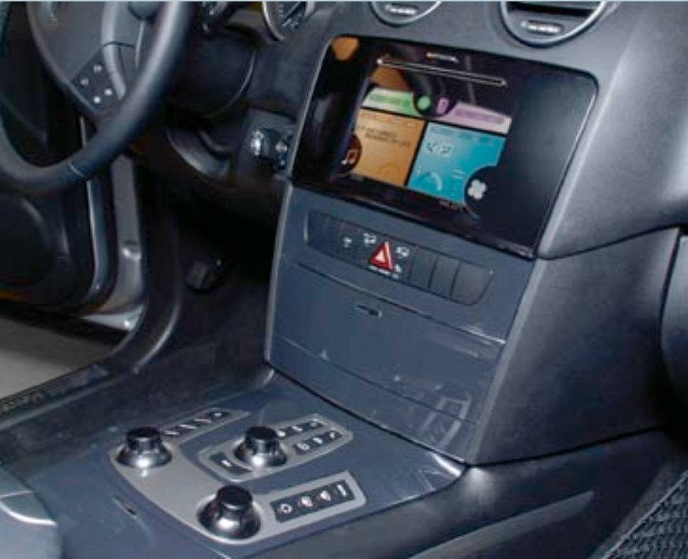
Graphical user interface for audio and air conditioning in the Valeo Demo Car.
