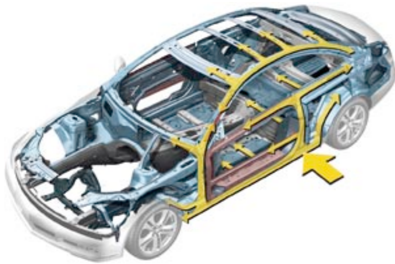
High strength of the roof pillars, the roof frame and the side longitudinal beams provide best protection of the passengers.
