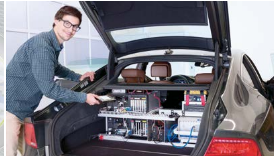
Test set-up for driver assistance systems.
