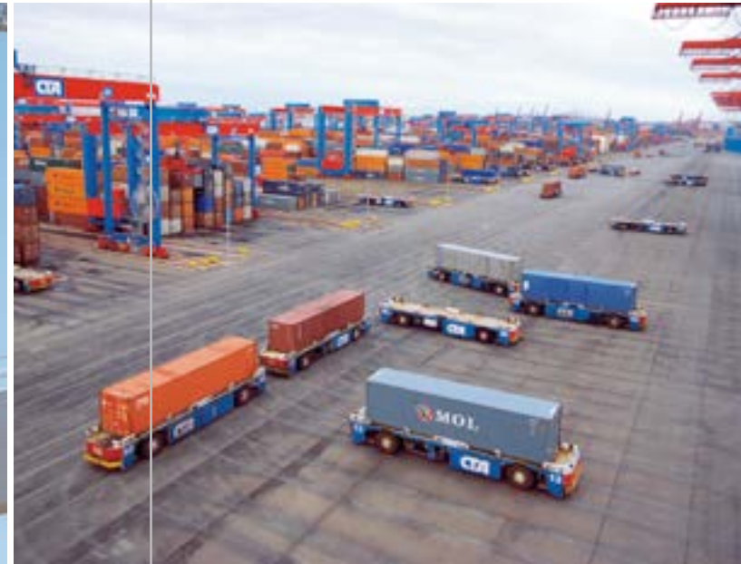
Automated guided vehicles transport containers at up to 6 m/s.
