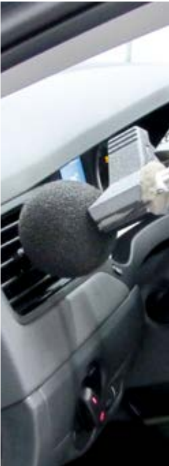
Near field measurement of the air vent
