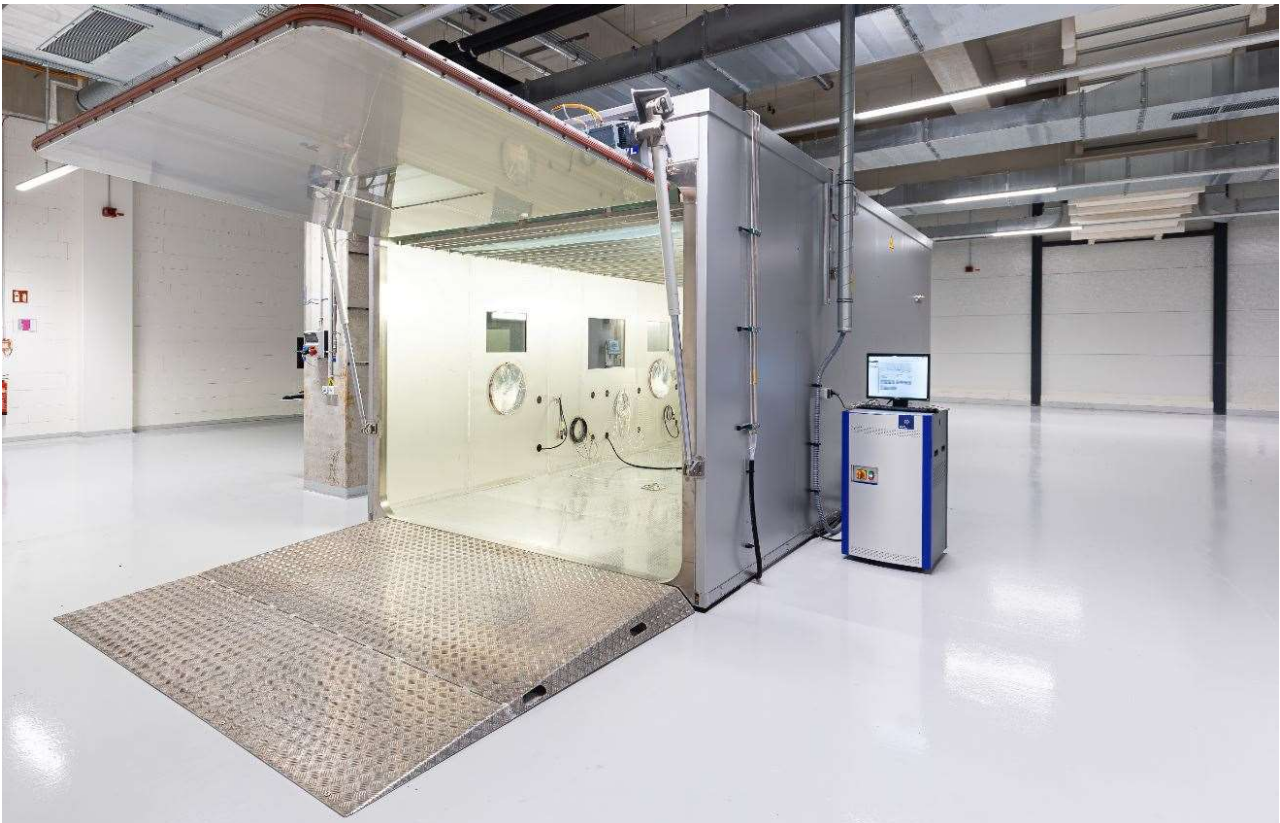
Kammer für Sealed Housing for Evaporative Determination Messungen (SHED)
